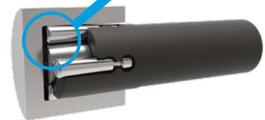
When setting the tool diameter above the nominal size of the tool then the taper will overlap the cage. Therefore the dimension "X" (see overleaf) will increase. This increase will be about 0.2 mm per 0.01 mm diameter enlargement (= one mark on the tool scale) of the tool setting.
