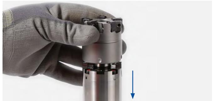
1. Clamp the milling cutter arbor in a changing device.
