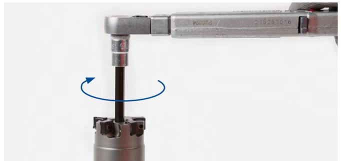
1. Adjust a torque wrench to the tightening torque required by the milling cutter manufacturer.
