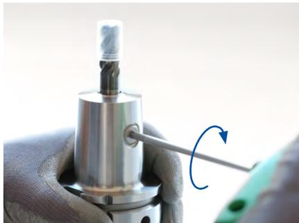
1. A torque wrench to the specified tightening torque (see Table "Tightening torques for the clamping screw").
