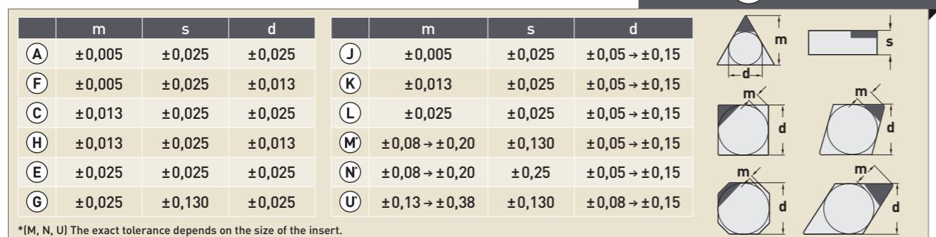
\***(M, N, U)** The exact tolerance depends on the size of the insert.
