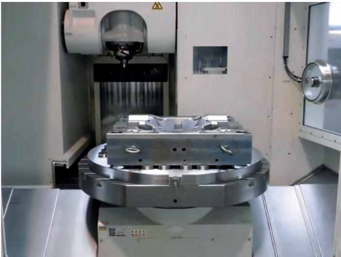
MillTec ROUND is the circular version optimized to be installed on 5-axis machines.
