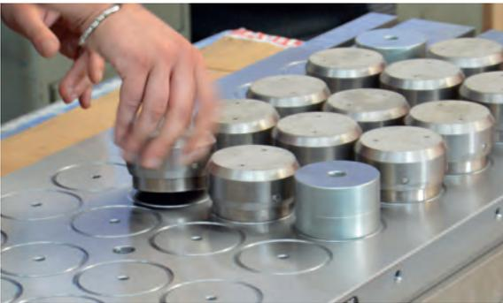
MILLTEC monolithic structure together with the RMP pole extensions create an extremely powerful clamping system for pieces on different heights or uneven surfaces, avoiding internal tensions in a simple and quick way.
