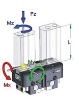
Clamping force diagram exterior gripping
