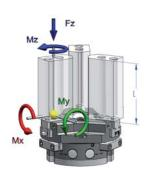
Clamping force diagram exterior gripping
