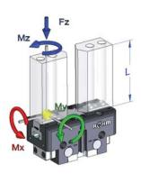
Clamping force diagram exterior gripping
