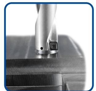
Paketbohren Bundle drilling
