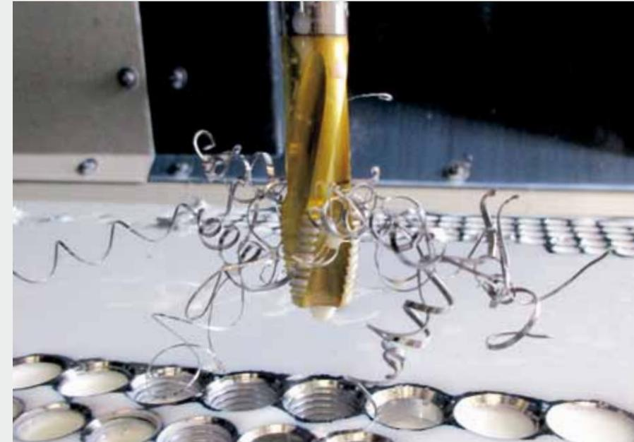
Small changes – increased impact: Thanks to the new chamfer at the top end of the ChipBreaker, the user avoids chip jams.
