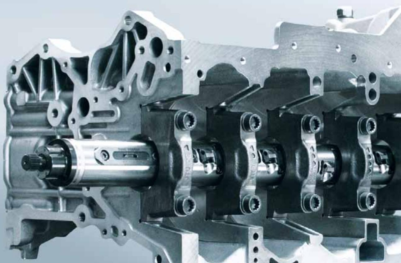
Wear to bearing boring bars is compensated by automatically controlled cutting edges. That generates, in addition to precision, a prerequisite for the Smart Factory.
