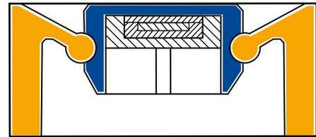
Chip in assembled state with fixing ring
