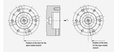
Spindle connection contour for adapter flange for short spindles in accordance with MN5000-13
