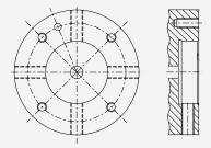
Spindle connection contour for adapter flange according to MN5000-12
