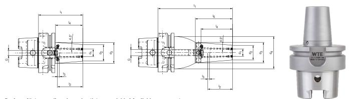
Design with two cooling channel outlets, resealable I Available on request
